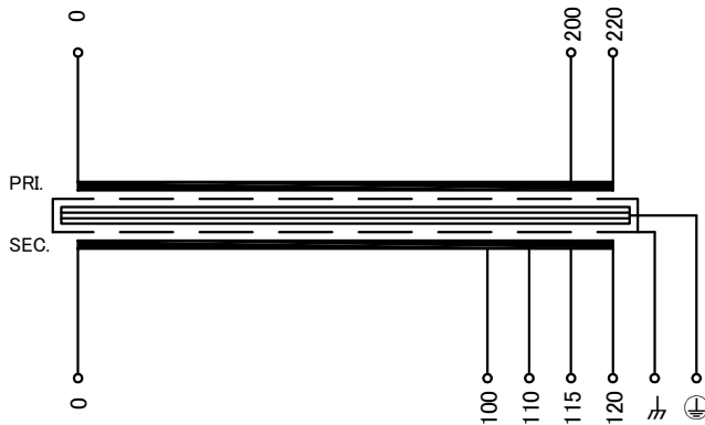
端子台配列 Terminal arrangement
